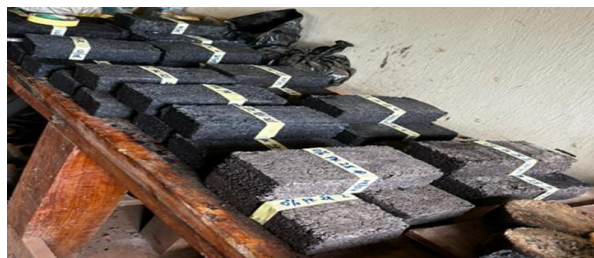
Plate 5: Polymer Interlocking Paver Blocks modified with various percentages of Nano-sized Palm kernel shells
